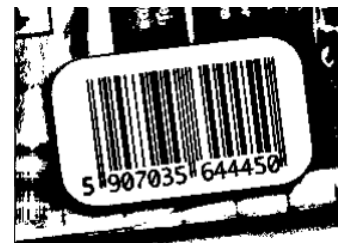
Result of ThresholdImage_Dynamic – the bars are correct.
