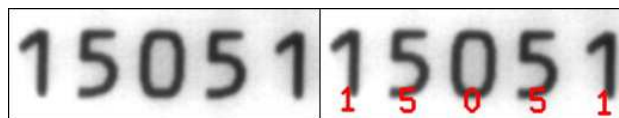
An example of optical character recognition using AvsFilter_DL_ReadCharacters tool. Left: The original image. Right: The image with the recognized characters drawn.
