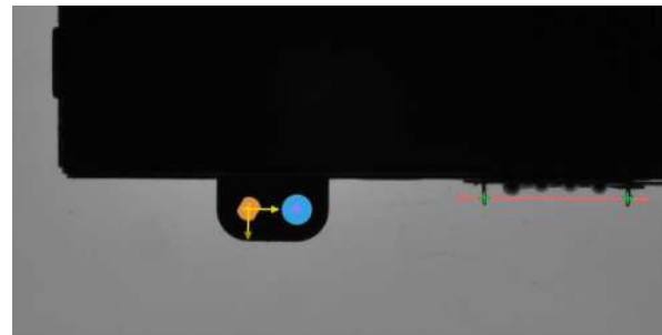
Created local coordinate system and an aligned measurement.
