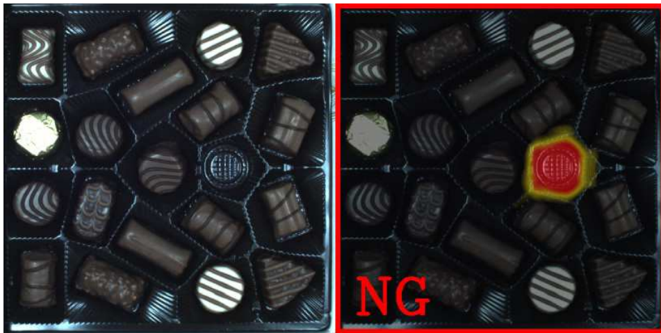
An example of a missing object detection using AvsFilter_DL_DetectAnomalies2 tool. Left: The original image with a missing element. Right: The classification result with a heatmap of anomalies.
