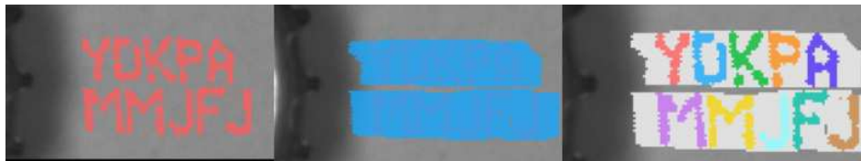
The process of splitting text into lines using region morphology filters.
